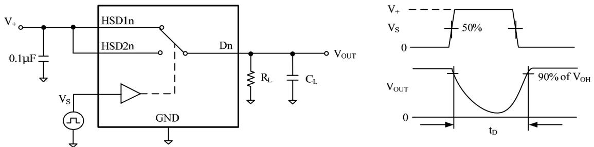
Test Circuit 3. Break-Before-Make Time ( $t_D$ )
