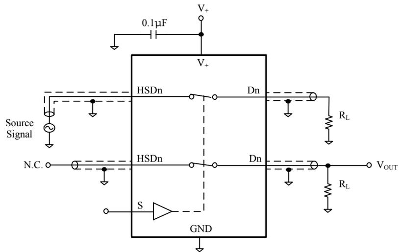
$$\text{Channel To Channel Crosstalk} = -20 \times \log \frac{V_{\text{HSDn}}}{V_{\text{OUT}}}$$
